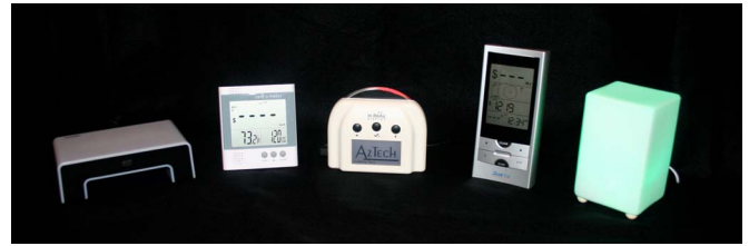
Fig. 1. In-home energy displays from left to right: Wattson, Cent-A-Meter, Aztech, PCM, and Ambient Orb.
